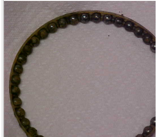
One of the old races with rusty ball bearings dry grease
